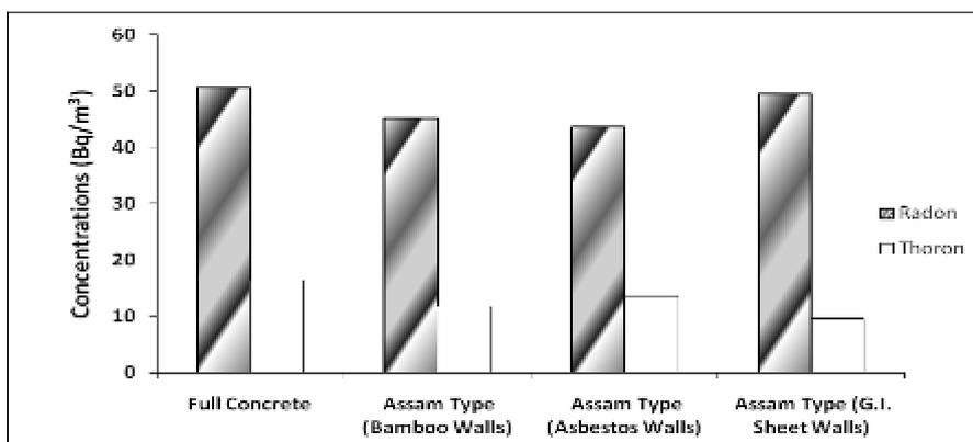
Figure 3. Correlation of radon/thoron concentration with construction types.
